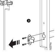
the left door by removing two (2) retaining screws and four (4) washers.
