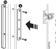
**6.** Install switch bracket **3** and left door bracket **0** onto left door, using two (2) screws from handle, removed in *Step 1*.
