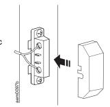
**4.** Use the black wood screw provided with the kit to attach the cable tie mount to right door.
