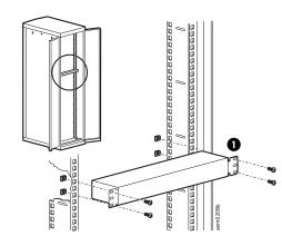
1. Ensure that the Rack Monitor 250 (NBRK0250) is properly installed in the NetShelter CX cabinet.
