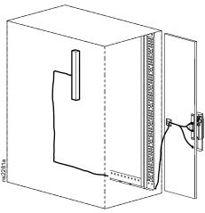
5. Route the door switch cable across the door. Near the hinge, direct the cable to the front bottom corner of the interior
