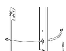
5. Feed the included cable assembly through the lock hole in the right door of the NetShelter CX.
