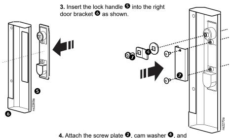
**4.** Attach the screw plate **②**, cam washer **③**, and new cam **⑦** from the NetShelter CX High Security Handle Adapter Kit.
